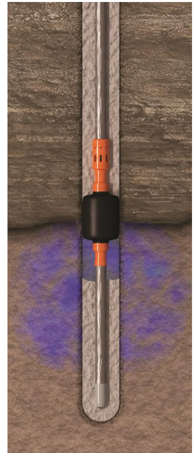
Casing Annulus Packer and Port Collar
