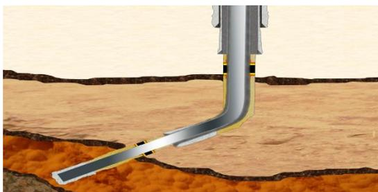
*FREECAP Swellable Packers provide Secondary annular barrier above hydrocarbon bearing zones in DeepWater GOM.*
