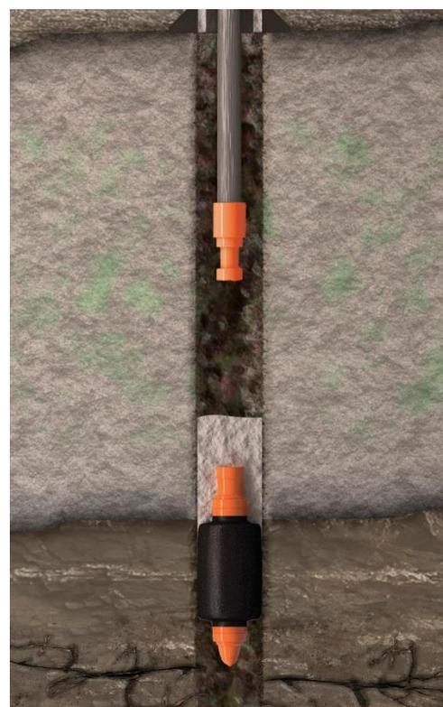
The TAMPlug Permanent Bridge Plug System isolates a lost circulation zone and allows the operator to regain control of the well.
