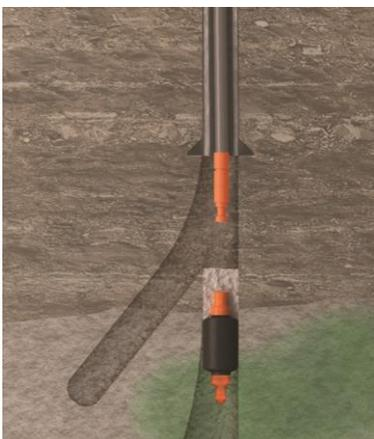
**RESULTS AND BENEFIT:** The TAMPlug was set successfully in the open hole, sealing off the gas below and allowing the operator to pump a cement plug without the concern of gas channeling through and around the cement. The operator could next pull out of the hole, pick up the drilling BHA, and kick off the plug. The lateral section of the well was then drilled successfully.
