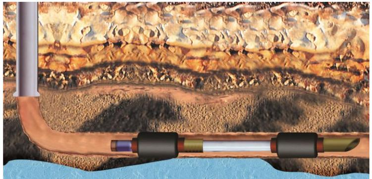
*FREECAP Scab Liner assembly successfully deployed for water shut-off*
